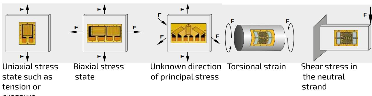
Different structural shapes for different applications
